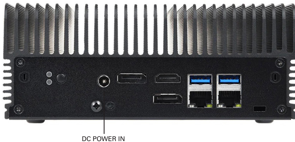
I/O CONTROL SIDE
