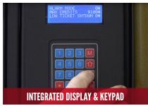
A new, larger LCD display offers improved messaging; a new 16-key keypad¹ adds integrated menu-driven navigation and provides local PIN sales capabilities.
